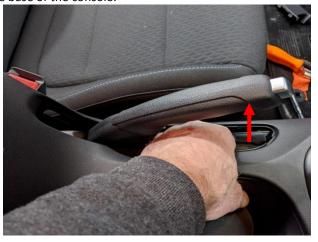
11. With both sides of the center section of the console loose, use your hand to tug straight up in the front area of where the shift boot was.
