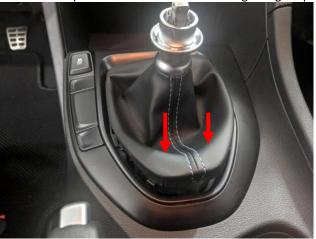
3. Open the center console and use a flat headed screw driver or a round point plastic pry tool to lift the edge of the console's passenger side molding.
