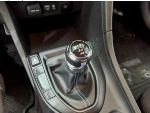
2. Wrap your fingers under the rear portion of the shift boot and tug straight up and remove the shift boot.
