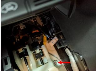
18. Perform the same steps as above with the 2 remaining rear bushings. Then, using a 12mm socket, tighten all 4 bolts.
