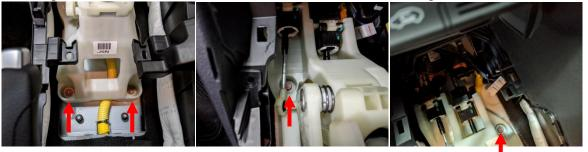
15. Using needle nose pliers remove all 4 metal sleeves and rubber bushings from the base of the shifter.
