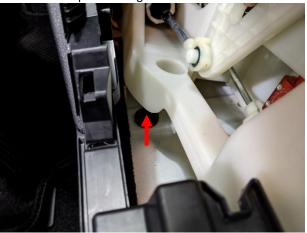
17. Next, from the top, slip the next shifter bushing under the front right so it indexes with the base of the shifter and install a bolt leaving it a bit loose.
