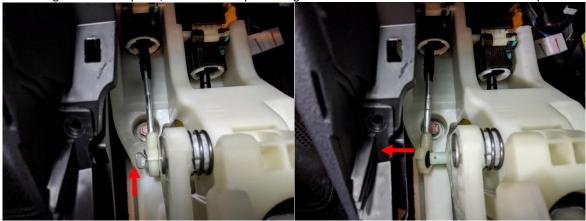
13. Using a philips head screw driver and a 10mm socket, extension and ratchet, remove the metal console support bracket.
