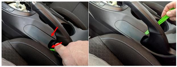
6. Using a flat head screw driver or pry tool, lift the passenger side of center section of the console to separate it from the center console storage box. Repeat for the driver's side.
