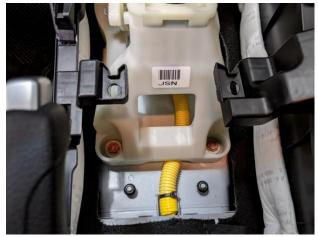
19. Replace the shifter cable and re-secure it with the clip removed in step 10.
