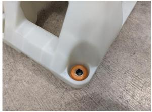
16. From the rear of the shifter base, go beneath the shifter base and place your first shifter bushing over the left front hole and lower the base carefully on to it so the male portion indexes with the base of the shifter. Install a bolt removed in step 14 leaving it a bit loose.
