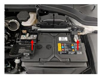
5. Using a 12mm socket, remove the battery hold-down bracket and remove the battery.
