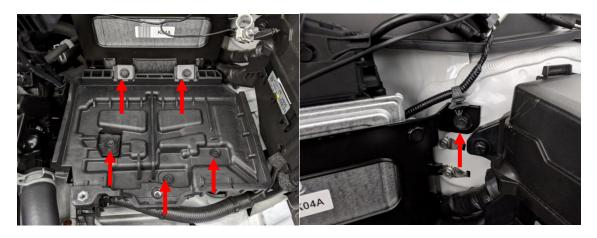
7. Remove the 2 connectors at the ECU. Then remove the ECU and battery tray from the vehicle.
