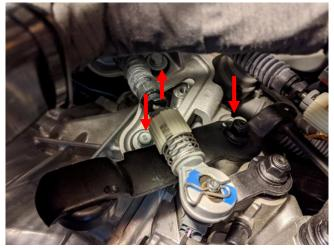
10. Remove the 3 metal sleeves and 3 rubber bushings from the mounting bracket.
