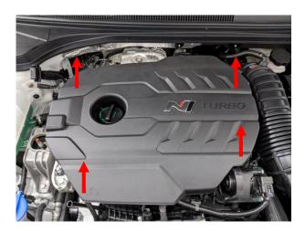
2. Using a pair of pliers and a 10mm socket, remove the 5 clamps securing the intake to the turbo, airbox, bypass valve hose and vacuum hoses. Remove intake hose from the vehicle.
