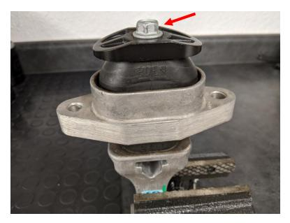
5. Disassemble the mount and re-assemble using your New JBR Lower Torque Mount Bushings.
