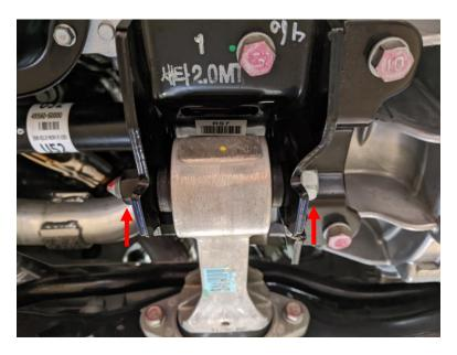
4. Lock the mount in a vice as shown below. Using a 14mm socket, remove the bolt securing the rear mounting flange.
