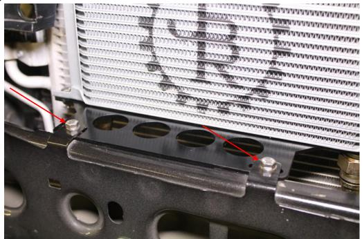
17. Using a 3/8" socket, install the nylon spacer behind the upper mounting bracket and use the hex head screw to complete the installation of the oil cooler core.
