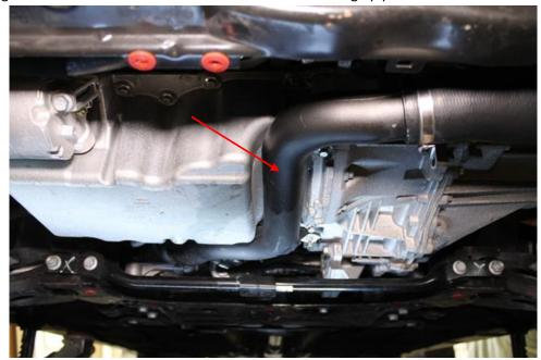
20. Slip the heat shielding covers over the braided lines in the area where they will near the lower radiator hose.
