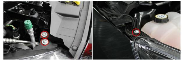
5. Carefully pull the bumper cover away from the fender on both sides.
