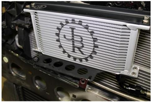
16. Secure the lower core mounting bracket to the tabs in the bumper support as far forward as possible.
