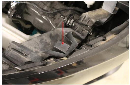
7. With the bumper cover pulled away, remove the fog light electrical connection on the driver's side and remove the front bumper cover assembly.
