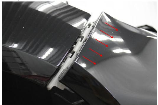
6. Press down to release the 2 clips found below where each headlight was. Then, begin slowly pulling the bumper cover away from the front of the vehicle.
