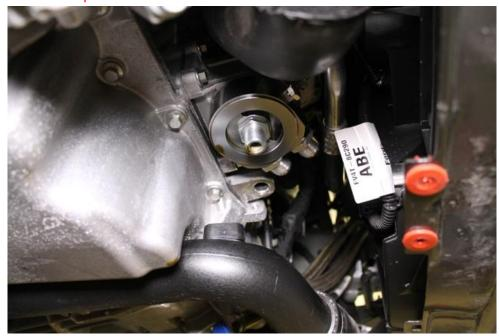
19. Using an 8mm and 10mm socket remove the hot side charge pipe.
