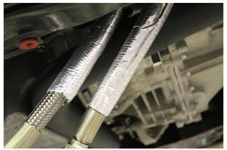
21. Route the hoses around the radiator core support and over the top of the lower radiator hose.
