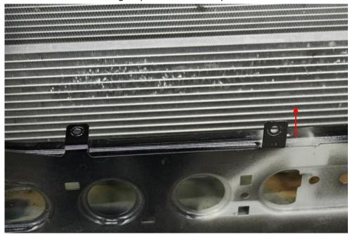
14. Start by slipping the lines behind the front radiator support.
