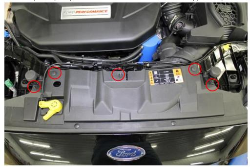
4. Using a T-30 torx, remove the 3 screws on both sides. Disconnect the electrical connections and remove the headlights.
