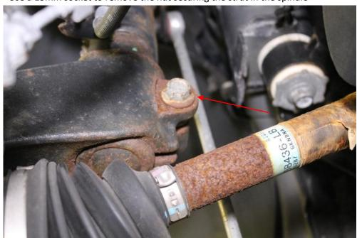
4. Using a large nosed chisel to spread the ears of the spindle and a large hammer if needed, push the spindle down and remove the strut from the spindle.
