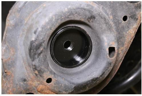
3. Transfer the rubber spring cover from the OEM spring over to your new JBR rear spring.
