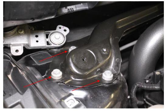
7. To remove the strut tower brace it will also be necessary to remove the 2, 10 mm nuts in the center of the engine bay as well as one at each wipe assembly.
