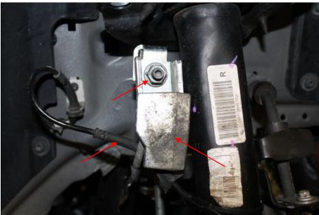
2. Using an 8mm socket remove the brake line.
