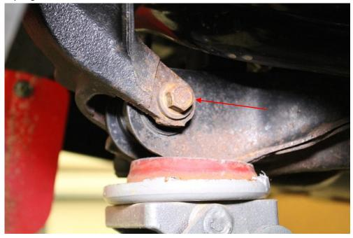
4. Install the rear spring perch as shown into the lower control arm. Thread the bolt and thick washer in from the bottom side and tighten to 70 ft/lbs.
