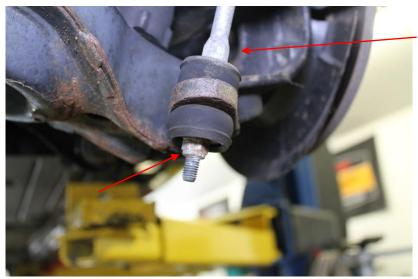
2. Use a 13mm socket and remove both nuts securing the upper shock mount and a 15mm socket to remove the lower shock mount.
