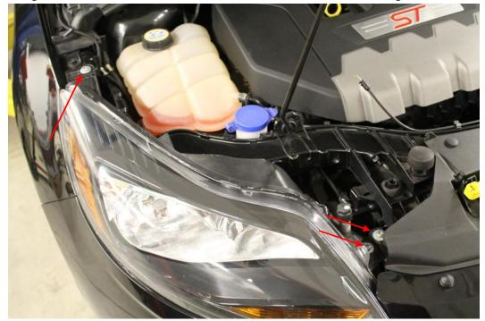
5. Remove the screws holding the front portion of the belly.
