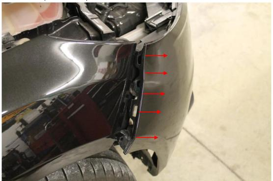
7. Press down to release the 2 clips found below where each headlight was. Then, begin slowly pulling the bumper cover away from the front of the vehicle.
