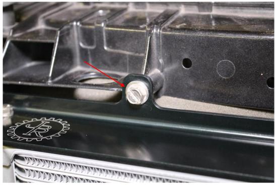
21. Secure the lower core mounting bracket to the tabs in the bumper support.
