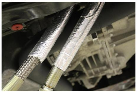
24. Route the hoses around the radiator core support and over the top of the lower radiator hose.
