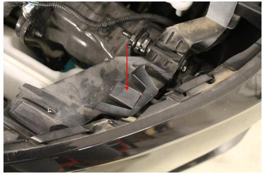
8. With the bumper cover pulled away, remove the fog light electrical connection on the driver's side.
