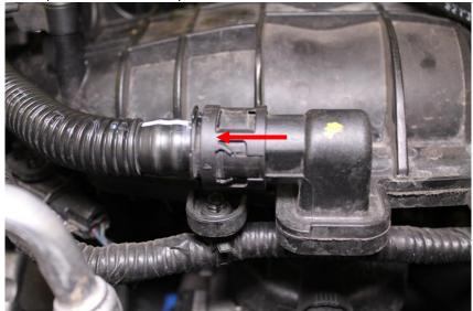
3. Remove the hose from the cam cover the same way.
