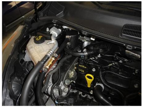
11. If you're installing your kit with a check valve, remove a 3" section of hose from the line leading to the intake manifold and install the check valve with the arrow point away from the catch can. Secure the hoses with the two clamps provided with your check valve kit.
