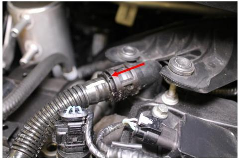
4. Remove the fastener securing the hose assembly to the timing cover
