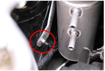
10. With the catch can now mounted, attach the long hose from the intake manifold to the top port on the catch can and the short hose to the bottom port and secure with 2 hose clamps and a flat head screw driver.
