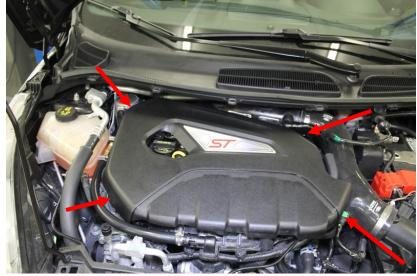
2. Using your right hand slide the color of the hose leading from the intake manifold towards the passenger side of the car and pull the hose off with your left hand.
