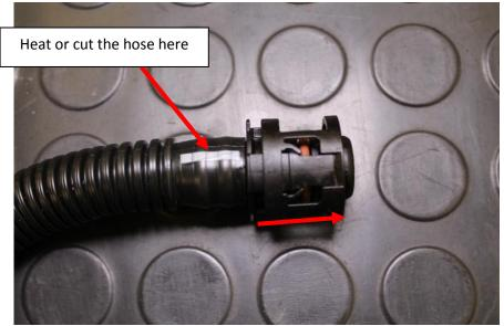
6. Reinstall both connectors and attach the 9" hose to the cam cover connector and the 24" hose to intake manifold and secure each with a hose clamp. Do not over tighten the clamps. Snug is all that's necessary.
