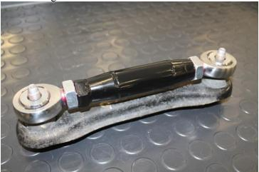
4. Lock the ends of the toe arm in place by tightening the jamb nuts on each end with a adjustable wrench.
