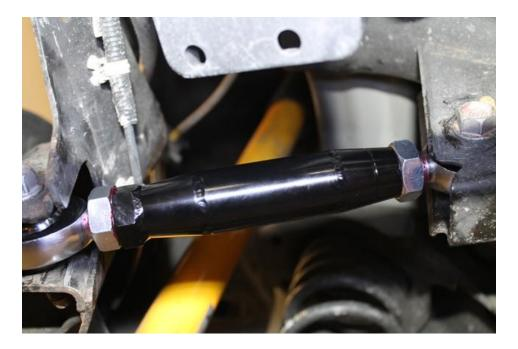
6. Now that the arms have been installed, both ends must be thoroughly covered in grease on both sides of the rod end. Failure to properly grease both sides of all ends after initial installation and at every oil change will cause premature wear and void the warranty.
