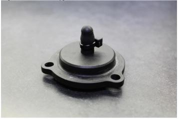
6. Replace the OEM bypass valve spring with the one included in your kit and assemble as shown. Then, re-install the assembly back into the vehicle.
