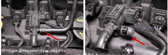
9. If installing a HKS or TIAL kit, install the valve onto your new JBR cold pipe now.
