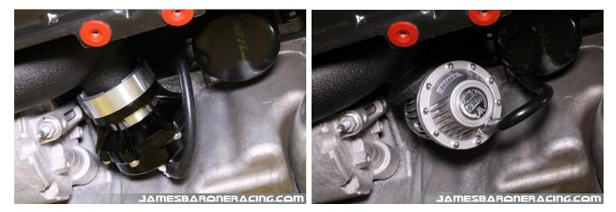
14. Orient the clamps for elbow as shown and tighten the clamps once all the adjustments are made and the fit is good.
