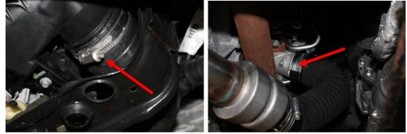
16. Using a 10mm and 13mm socket, remove the two bolts that secure the metal portion of the OEM charge pipe to the motor. One is located at the front and one at the rear of the oil pan. Remove the entire assembly as one unit.
