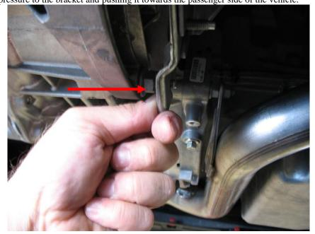
5. Using a 15mm socket remove the horizontal bolt that secures the motor mount to the transmission.
