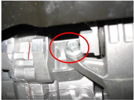
9. Using a 15 and 17mm wrench remove the nut securing the end link to the sway bar on both sides.
