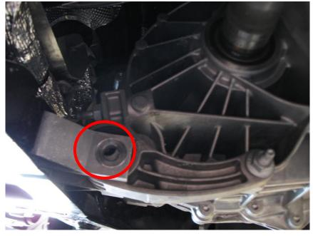
6. Using a 15mm socket remove the vertical bolt that secures the motor in the sub-frame.
