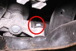
14. Using an 18mm socket and a 21mm socket remove the 4 bolts that secure the sway bar brackets to the top side of the sub-frame. Lower the sub-frame and remove the front sway bar.
