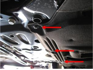
3. Once the belly pan is removed and the rear mount is exposed, remove the 6 nuts shown below that secure the down pipe support bracket to the transmission with a 13mm socket.
