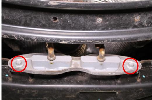
11. Remove the rear sub-frame cross brace using a 15mm socket. Support the sub-frame with a jack or jack pole. Remove 8 bolts using a 13, 15, and 21mm socket. A long extension should be used through the hole in the lower control arm to access the front sub-frame bolts.
