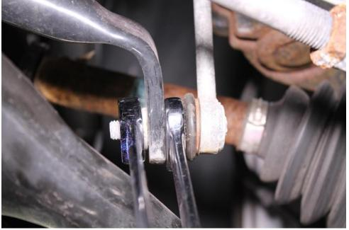
10. Using a 10mm socket remove the two bolts that hold the down pipe bracket to the sub-frame.
