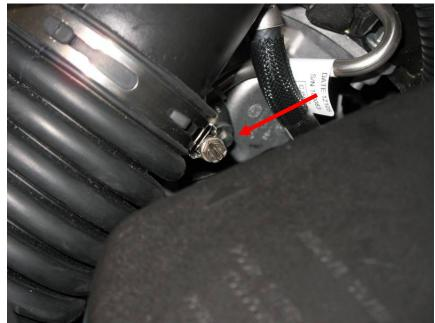
6. Disconnect the MAP sensor connector by squeezing the tab while pulling towards the passenger side.
