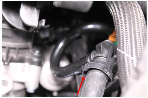
18. Connect the hose with the  $90^{\circ}$  fitting on to the port on the manifold.
