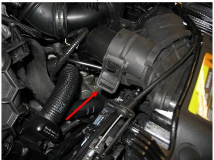
8. Now that everything is disconnected it's time to remove the entire air box assembly. There are 3 pegs that secure the air box to the vehicle. Below is the location of each of the grommets that the pegs fit in shown after the air box has been removed. Locate the pegs and pull the air box straight up in each area to pop the pegs out of their grommets and remove the entire assembly carefully.
