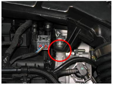
5. With an 8mm socket, loosen the clamp securing the intake hose to the turbo inlet pipe.
