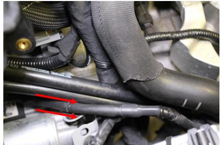
20. Connect the hose attached to the back of the intake manifold to the OUT port on the catch can. Secure it using one of the hose clamps provided with your kit and a flat head screw driver. Connect the hose from the PCV valve to the IN port on the catch can.
