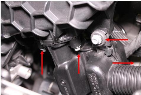
15. With the sound symposer out of the way we need to remove the PCV hose connection at the manifold. This can easily be done with both hands by reaching in behind the manifold from the driver's side. Use your right hand to squeeze both sides of the connector together. Use your pointer finger on your left hand to push it off towards the rear of the car. The next 3 pictures illustrate how to grab the connector and position yourself to get it off. It may take a few tries; be patient here.
