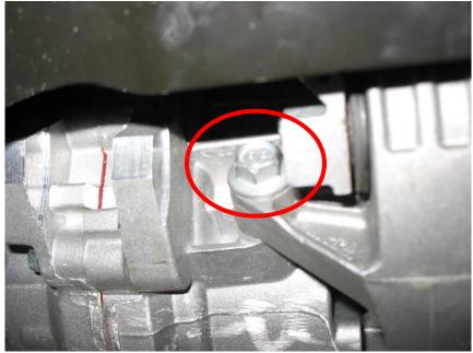
9. With the OEM motor mount now removed, install your new JBR rear motor mount. The mount may fit snug and be tough to move in the sub-frame. Apply some dish soap to both sides of the bushing to make it slide in and move around easier. Push the mount deep in to the sub-frame. Reinstall the motor mount bracket; all three bolts remove in steps 7 and 8 and torque to 45 ft/lbs.
