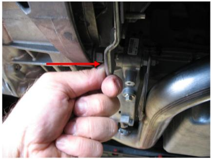
5. Using a 15mm 6-point socket remove the horizontal bolt that secures the motor mount to the transmission.
