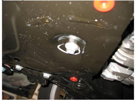
7. Push the OEM mount towards the rear of the vehicle deep in to the sub-frame then with a15mm closed end wrench remove the 2 bolts shown below that secure the motor mount bracket to the transmission. The motor may need to be pivoted towards the front to remove the rear most bolt.
