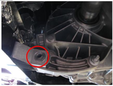
6. Using a 15mm 6-point socket remove the vertical bolt that secures the motor in the sub-frame.
