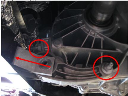
8. With a15mm closed end wrench remove the 3<sup>rd</sup> and final bolt that secures the motor mount bracket to the transmission and remove the bracket and the motor mount.
