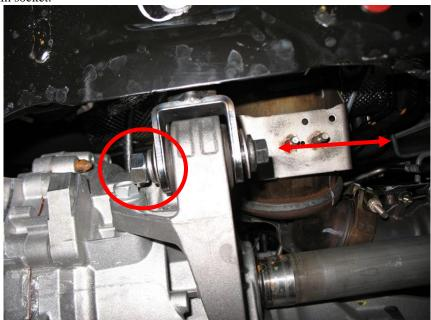
11. Install the vertical bolt removed in step 6. You may need to pivot the motor again to install the bolt. Torque to 70 ft/lbs.
