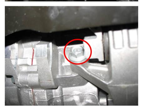
10. Next place the flat washer included with your mount on to the horizontal bolt removed in step 5 and install the bolt through the mount and transmission bracket. Put another flat washer, then a lock washer and the nut supplied with your mount on to the bolt. You may need to back the bolt out of the mount a bit towards the driver's side in order to get the nut on. Tighten by hand first then, torque to 90 ft/lbs. with a 19mm open ended wrench and a torque wrench with a 6-point 15mm socket.
