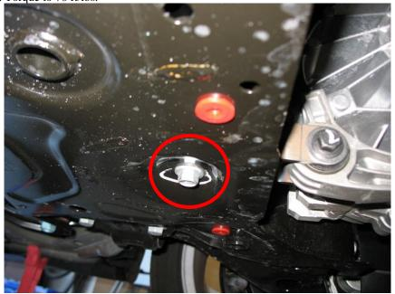
12. Reinstall the downpipe support bracket, tighten all 6 nuts and reinstall the belly
