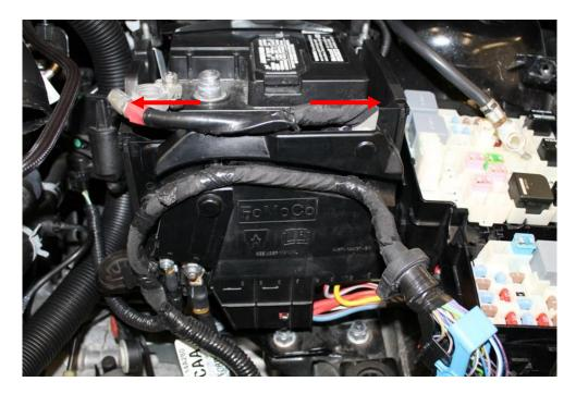
15. Slide the battery forward and remove the electrical connector at the negative terminal and remove the battery from the vehicle.
