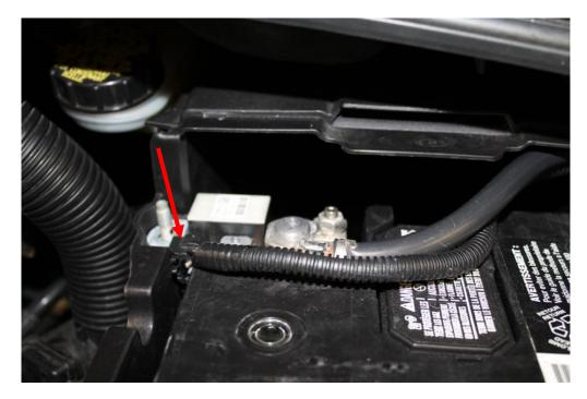
16. Using a 10mm socket, remove 3 bolts securing the battery box and remove the battery box and sound symposer assembly from the vehicle.
