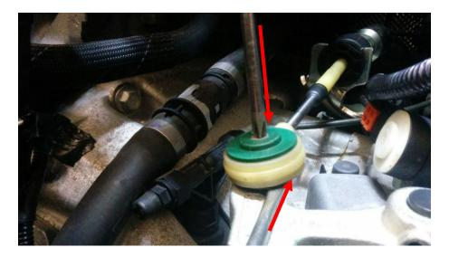
18. Remove both cables from the mounting bracket by sliding the knurled portion of the cable jacket back towards the rear of the car and lifting up out of the bracket.
