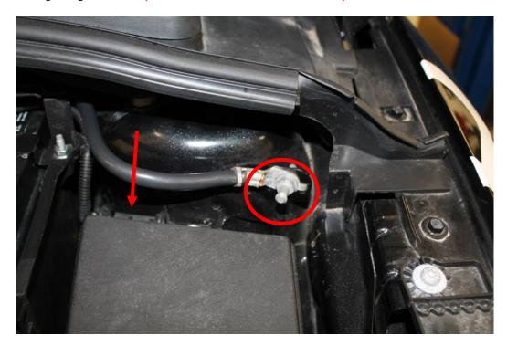
12. Using a 10mm socket, remove the positive battery cable and the battery hold down strap.
