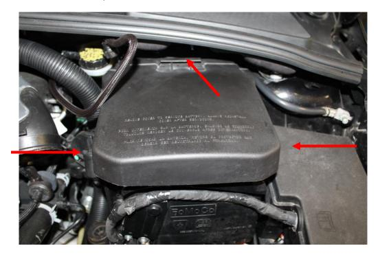
11. Remove the fuse box cover by depressing the tab at the rear of the cover. Using a 13mm socket, remove the negative ground wire. (BE SURE IT TOUCHES NOTHING METAL)
