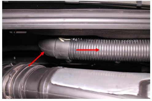
4. Install the cap provided with your kit in to the hole in the firewall.
