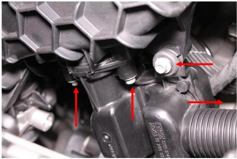
2. Using a T20 torx bit, remove the screw securing the symposer valve to the battery box and pull the hose off. Also, remove the hose between the intake and the valve at the battery box.
