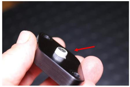
6. Insert the o-ring supplied with your kit in to the groove in the symposer block-off plate.
