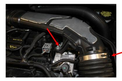
4. Squeeze both sides of the vacuum connector shown below and remove.
