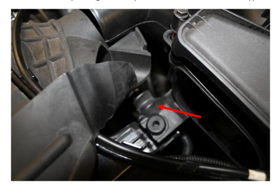
7. Remove the MAP sensor connection by depressing the tab and pulling towards the passenger side.
