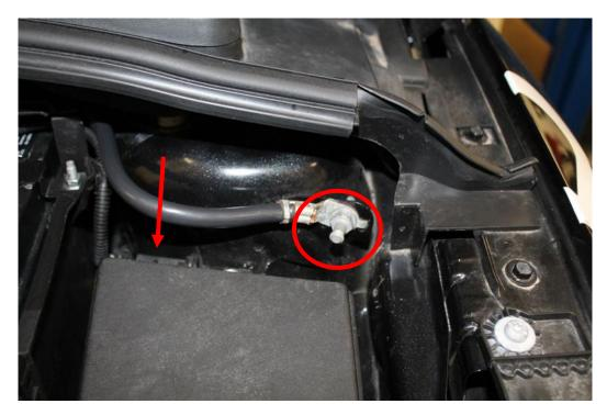
14. Using a 10mm socket, remove the positive battery cable and the battery hold down strap.
