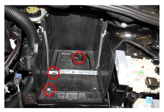
20. Using a 14mm socket, remove the 4 nuts securing the battery box mounting bracket. Then using a 19mm socket, remove the main center bolt from the transmission mount and remove the upper half of the OEM mount from the car.
