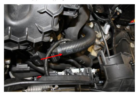
10. Remove the electrical connector from the sound symposer control module by depressing the tab and pulling down..
