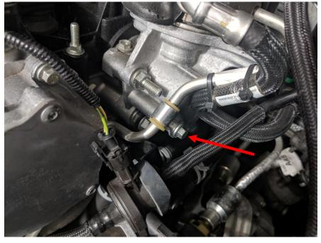
16. Install the mounting bracket included with your kit. (Be careful not to cross-thread this bolt when reinstalling) Leave the bolt just a little loose.
