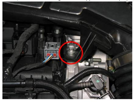
5. Using an 8mm socket remove the bolt securing the turbo inlet pipe to the valve cover and a 12mm wrench to remove the peg that supports the engine cover.
