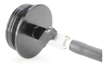
8. Apply Teflon tape to the threads of the barbed fittings. Install the barbed fittings into the IN and OUT ports of the catch can using a 14mm deep socket.
