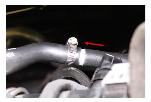
20. Connect the hose with the female quick connector to the back of the valve cover with the elbow of the connector pointing almost straight down.
