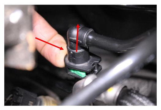
13. Now swivel the fuel line towards the passenger side and secure it to the hard line with the included zip tie. Put the green clip removed in step 16 back on the vacuum line connector and reconnect the vacuum line.
