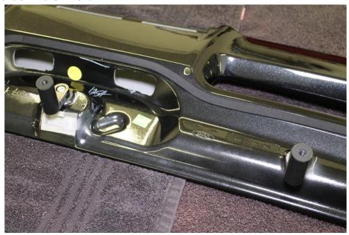
5. Install the 2 medium and 2 small wing risers, oriented as shown below to the wing using 4 #6 x 3/4" stainless screws. Snug but do not tighten with a philips head screw driver.
