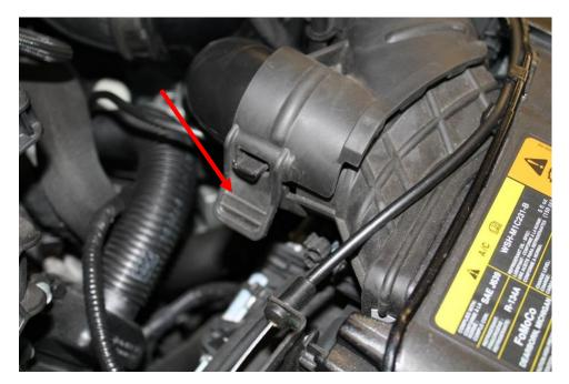
4. Remove the rubber strap securing the bottom portion of the air box to the front core support.
