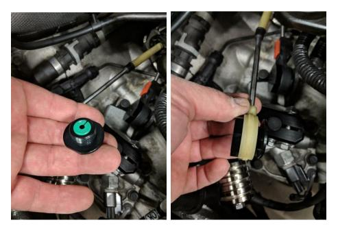
13. Slip the female half through the cable and thread the two together. Tighten by hand.
