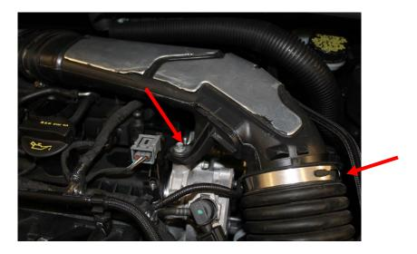
2. Squeeze both sides of the vacuum connector shown below and remove.
