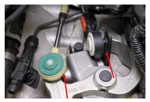
8. Using a medium screw driver, pry between the cable head and the plastic collar breaking it off. Then, remove the bushing from the end of the cable.
