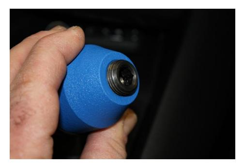
8. Carefully thread the shift knob on to the adaptor. It may be necessary to remove the knob and make small adjustments to the jamb nut inside the knob to close the gap between the shift boot and the base of the shift knob and for it to stop in about the 11 o'clock position shown below.
