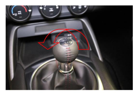
6. Using a 15mm 6 point socket carefully install the included shift knob adapter on to the shifter stalk until it's all the way down to where the threads stop and tighten to 12ft-lbs.
