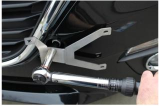
7. Using a 10mm socket and 10mm socket wrench, attach your license plate to the Toe Tag using the 4-10mm bolts, 8-flat washers and 4-10mm nyloc nuts.
