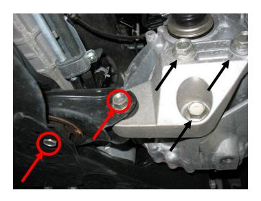
3. Remove the old motor mount; put your new JBR Chrome-Molly mount in place and install the
