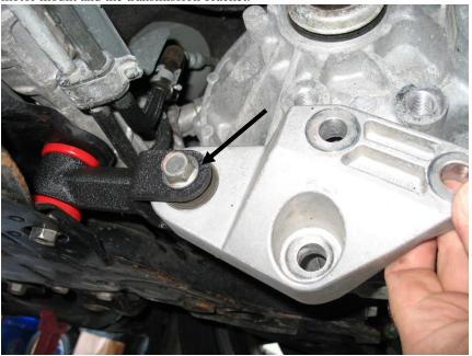
5. Pivot the transmission bracket up in to place and install the 3 bolts previously removed. Rocking of the engine may be required to align the bolts. Using a 19mm socket, socket wrench and torque
