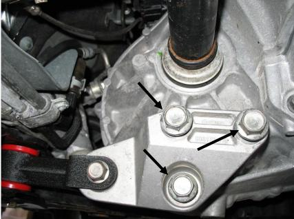
6. Put the supplied lock washer and nut on to the bolt. Tighten and torque to 70 foot-pounds using a
