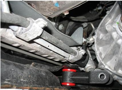
4. Put the transmission bracket into position as shown below and slip the mounting bolt through the motor mount and the transmission bracket.
