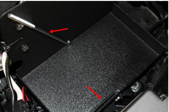
9. Place your 51R battery in to the tray, put the hold down hooks through the holes in the hold down bar and secure each hook with a flat washer and a lock nut. Then tighten down the bar with a 10mm deep socket. Now, reconnect the positive battery terminal first then the negative terminal.
