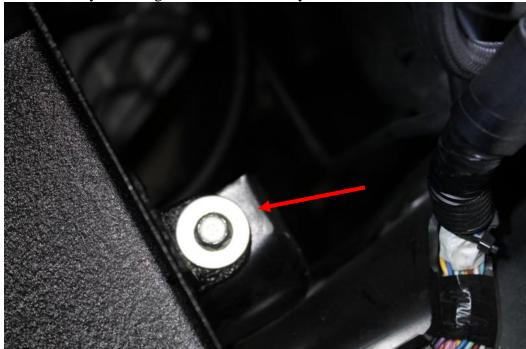
7. Using the included stainless bolt, two flat washer and lock nut, secure the passenger side of the battery box and tighten with a 10mm socket and 10mm
