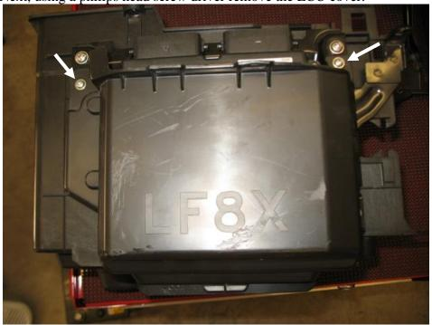
3. With the cover removed, now remove the 4-10mm ECU mounting nuts, remove the ECU from the factory battery box and save the nuts for later use.
