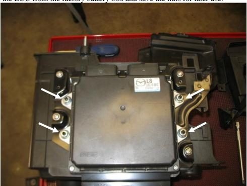
4. Remove the metal ECU wiring harness mounting bracket by pulling the tab shown below towards you and pulling the bracket towards the rear of the car. Remove the bracket from the vehicle.
