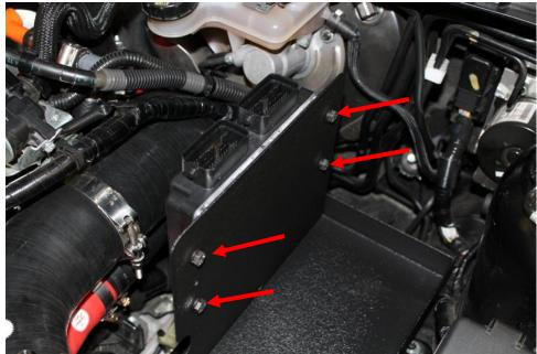
7. Reconnect the harness to the ECU and use the included zip tie to secure the
