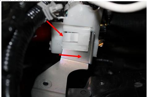
5. Disconnect the ECU wiring harness from the mounting bracket securing it to the transmission. Push the tab shown below towards the rear of the car pull up.
