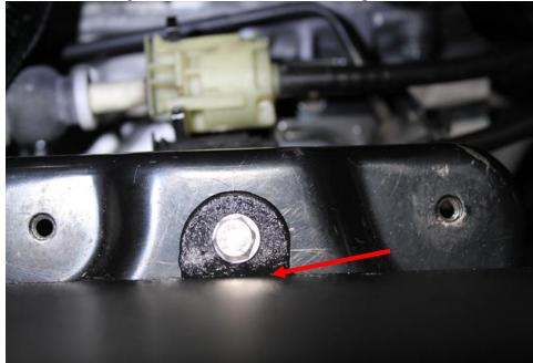
8. Next place 1 black nylon washer on each of the remianing 4 bolts include with your kit. Place two of them through the rear ECU mounting holes on the battery box and hold them in place with 2 fingers. Put two more black nylon washers on the bolts, and then put the ECU on to the two rear bolts. Use 2 of nuts removed in step 3 and loosely secure the ECU. Repeat for the front two mounting holes and then tighten all four with a 10mm socket and 10mm wrench.
