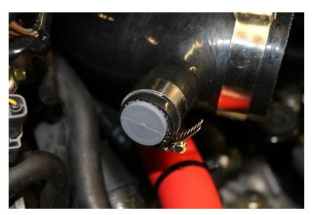
12. Next, feed the other hose removed in step 7, down in front of the EGR valve, underneath the bypass hose and connect it to the cam cover vent with a hose clamp. This can be done without removing the battery box. The picture below illustrates the routing if the battery box and turbo inlet pipe was removed.
