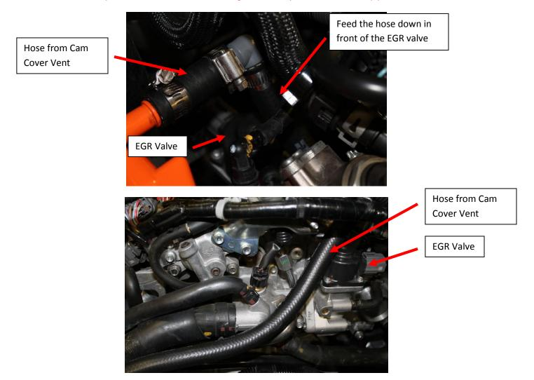
13. Loosely secure the hose from the Cam Cover to the bypass hose and/or the radiator hose so it doesn't interfere with the shifter linkage.
