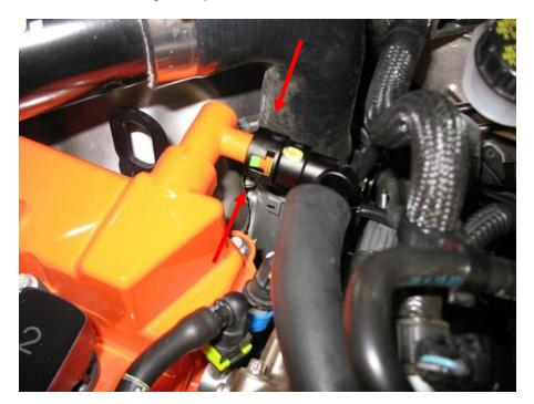
10. Loosen the clamp on the intake hose and remove the OEM Cam Cover hose
