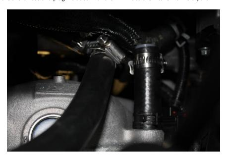
10. Remove the OEM hose from the CAM cover by squeezing the 2 green tabs and pulling the hose off of the cam cover. Then, remove the green clip from the Cam Cover.
