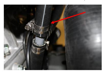
9. Attach the short hose and plug included with the VTA kit to the intake manifold port.
