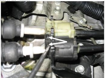
13. Remove the 2 x 17mm nuts and 1 x 17mm bolt from the transmission perch and remove the perch from the vehicle. Be careful not to damage the shifter cable when removing the forward most nut.
