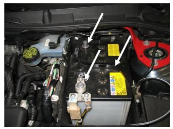
3. Using needle nose pliers, remove the 3 cable connectors from the front panel of the battery box. Remove the front panel of the battery box by sliding it up, then remove the battery.
