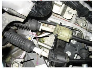
14. Install the new JBR transmission perch in the vehicle. Using 3 of the supplied lock washers and the short bolt also supplied, torque to 60 foot pounds. Then put the shifter cable back in to the mounting bracket and push down until it snaps in to place.
