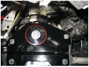
17. With the perch installed place the thick washer over the stud and on to the perch.
