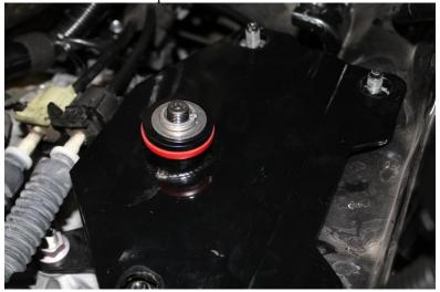
19. Remove the jack supporting the transmission to allow the transmission mount to settle in to place.
