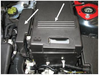
2. Remove the 2 x 10mm nuts from the battery hold down bracket, remove the negative batter cable and then the positive battery cable. Always remove the negative battery cable first and replace it last.
