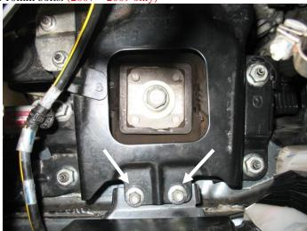
10. Remove the 4 x 17mm nuts and the battery box support bracket that covers the factory transmission mount. (The 2007 – 2009 models have anti vibration weight located towards the rear of the vehicle that will be removed as well)
