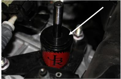
18. Install the transmission mount over the stud on to the perch. Make sure the mount is sitting flush on the perch. Place the other thick washer over the stud first, then the flat washer, then the lock washer. Thread on the nut and torque to 65ft/lbs.
