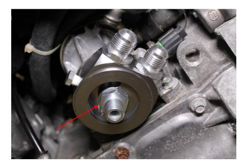
15. Using a pair of pliers, remove the clamp securing the coolant hose leading to the OEM oil cooler. Then, insert a flat head screwdriver into the metal fitting and carefully bend the fitting towards the front of the vehicle about a ½". It will move very easily. Reconnect the hose when finished.
