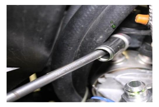
16. Using two 6mm x 35mm bolts, two flat washers and two spacers, install the oil cooler core, hose and mounting bracket assembly where the two bolts in step 13 were removed as shown below. Tighten the two bolts with a 10mm socket.
