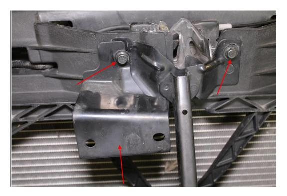
12. Again, using a 10mm socket, remove the bolt securing the sensor to the angle bracket and the two bolts securing the bracket to the top of the OEM crash bar.
