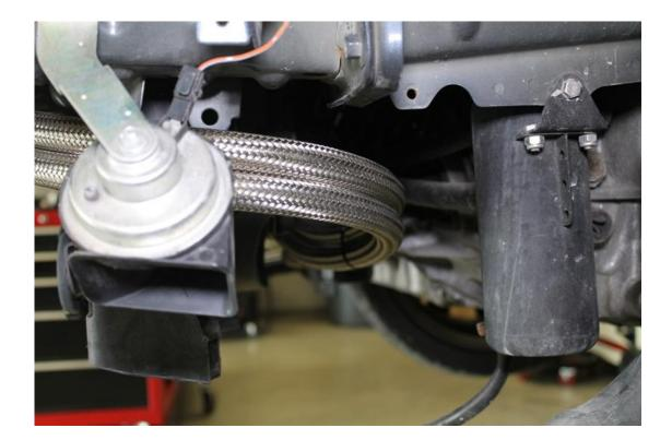
19. Slip the heat shielding covers over the braided lines and place in the area near the lower radiator hose and behind the radiator.
