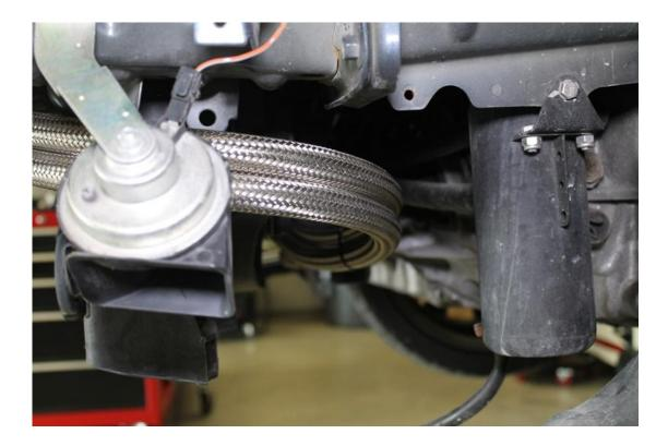
18. Slip the heat shielding covers over the braided lines and place in the area near the lower radiator hose and behind the radiator.
