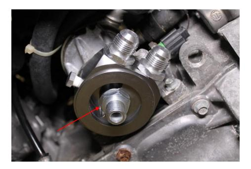
14. Using a pair of pliers, remove the clamp securing the coolant hose leading to the OEM oil cooler. Then, insert a flat head screwdriver into the metal fitting and carefully bend the fitting towards the front of the vehicle about a ½". It will move very easily. Reconnect the hose when finished.
