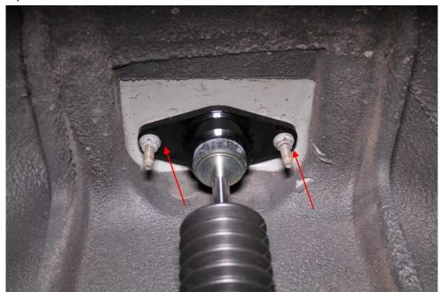
9. Using a jack, raise the lower control arm enough to put some pressure on the rear spring and to keep the rear spring seated if it's a bit loose. Adjust the rear shock until the lower bolt lines up. Tighten the lower shock bolt to 45-50 ft/lbs.
