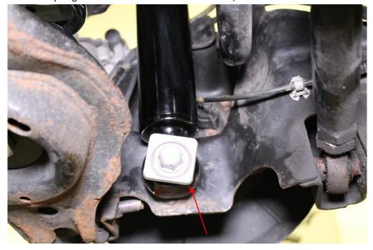
10. Now that the shock is secured both top and bottom, tighten the locking collar with the spanner wrench.
