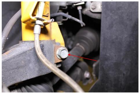
4. Remove the ABS sensor connector then spray some penetrating oil on top of the spindle where the strut is inserted.
