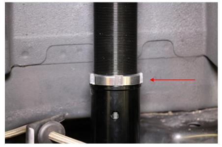
11. Remove the panels of the rear hatch or trunk area to gain access to the tops of the shocks. Insert the 12" rear adjustment keys in tops of the shock shaft and route to a place that's accessible and convenient for you to adjust the dampers.
