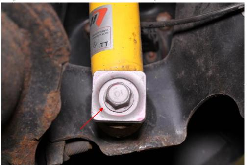
4. Support the rear lower control arm with a jack. Use a 17mm socket to remove the bolt securing the control arm to the spindle. Lower the jack slowly and remove the OEM spring.
