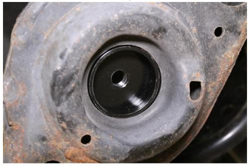
6. Transfer the rubber spring from the OEM spring over to your new JBR rear spring.
