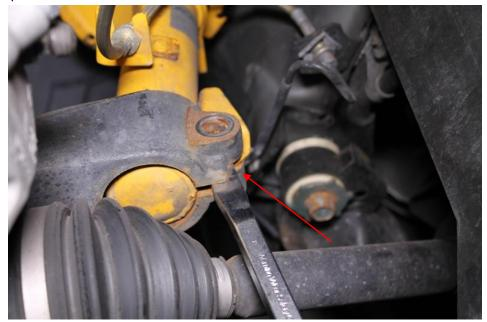
6. Use a hammer to knock the spindle down and remove the lower portion of the strut from the spindle.
