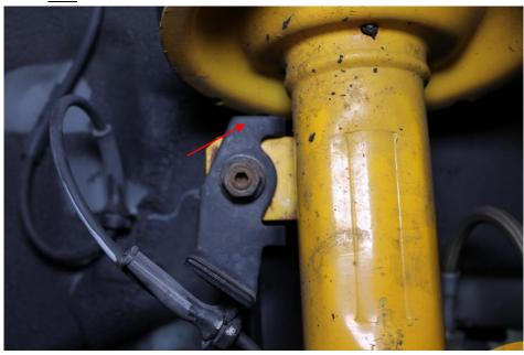
2. Using a pair of pliers remove the front brake line clip.
