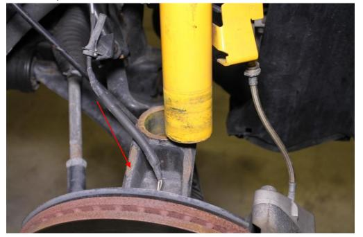
7. Remove the 3 upper strut mounting nuts using a 14mm socket and remove the strut & spring assembly from the vehicle.
