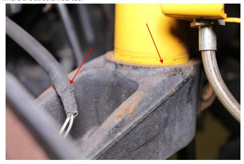
5. Drive a chisel in between the ears of the spindle to open and release the strut from the spindle.
