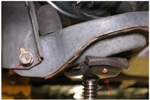
5. Install the rear spring perch as shown into the lower control arm. Thread the bolt and thick washer in from the bottom side and tighten to 70 ft/lbs.
