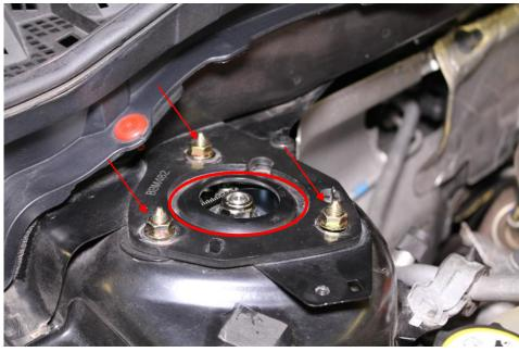
9. Spray WD-40 in to the spindle and insert the lower portion of the JBR coilover, properly indexing the tab between the ears, then into the spindle. Use a jack or jack pole to raise the spindle until it's seated. Secure with the bolt removed in step 3 and tighten to 40-45ft/lbs. Re-install the brake line and clip as shown and tap in place with a hammer
