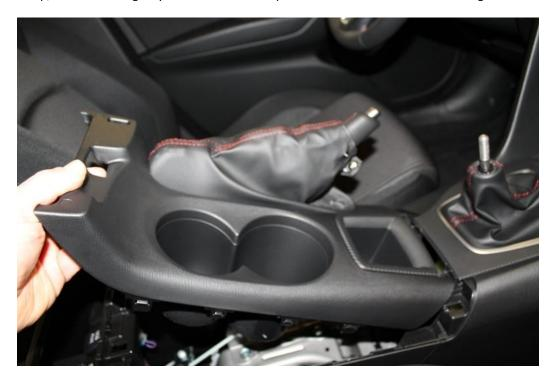
5. Lift up and slightly and pull to remove the section surrounding the shifter. The section in front of the shifter may come with it.
