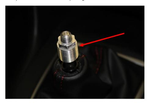
9. Next thread the jamb nut in to the shift knob using a 3/8" allen wrench or large flat head screw driver until it bottoms. Then, back the jamb nut out 6 full revolutions.
