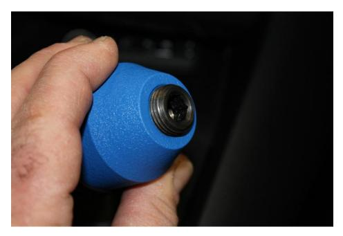
10. Carefully thread the shift knob on to the adaptor. It may be necessary to remove the knob and make small adjustments to the jamb nut inside the knob for it to stop in about the 11 o'clock position shown below.
