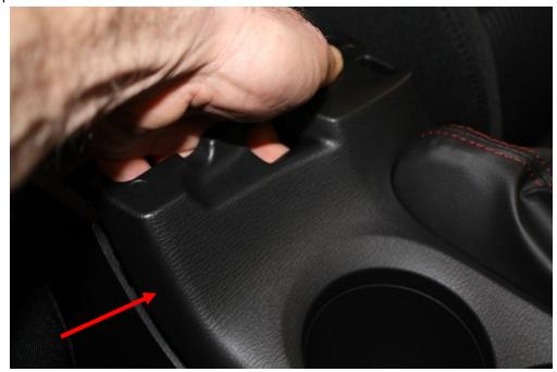
4. Lift up, clear the emergency brake handle and separate it from the section surrounding the shifter.
