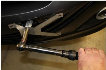
5. Using a 10mm socket and 10mm socket wrench, attach your license plate to the Toe Tag using the 4-10mm bolts, 8-flat washers and 4-10mm nyloc nuts.
