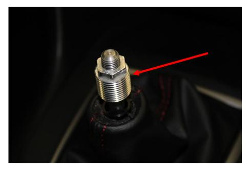
7. Next thread the jamb nut in to the shift knob using a 3/8" allen wrench or large flat head screw driver until it bottoms. Then, back the jamb nut out a full 2.75 revolutions.
