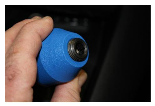
8. Carefully thread the shift knob on to the adaptor. It may be necessary to remove the knob and make small adjustments to the jamb nut inside the knob for it to stop in about the 11 o'clock position shown below.
