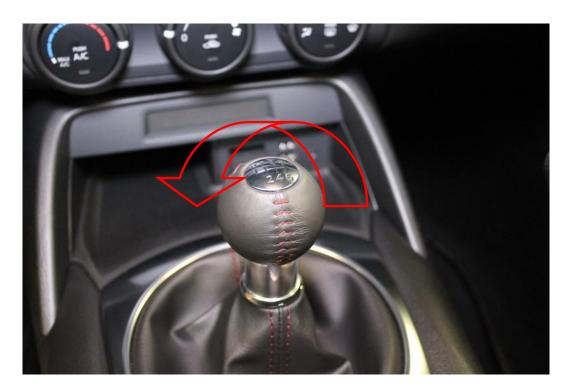
6. Using a 15mm 6 point socket carefully install the included shift knob adapter on to the shifter stalk until it's all the way down to where the threads stop and tighten to 12ft-lbs.
