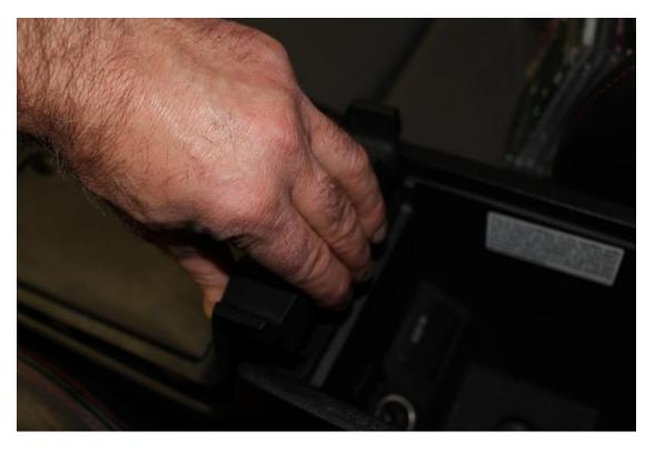
4. Remove the cup holder and shift boot portion of the console together or separately if they've come apart in two pieces.
