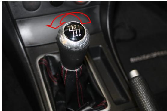
2. Loosen the shift boot portion of the console by crabbing it under the edge of the silver trim ring and pulling up.
