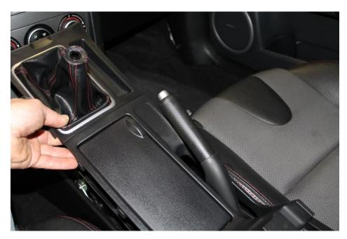
5. Place the two Philips head screws through the holes in the gate guard and lower it in to place just to the driver's side of the shifter.
