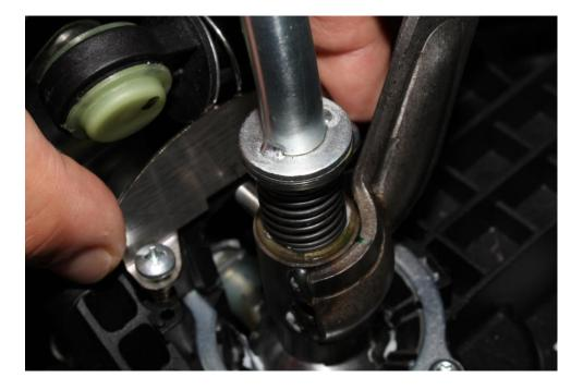
6. Using a Philips head screw driver tighten each of the screws to secure the gate guard in place.
