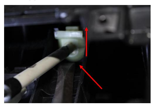
8. Using a large screw driver under the lip of the cable attachment clip, pop the left cable attachment clip up to remove it from the shifter base.
