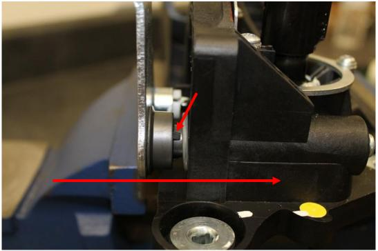
22. Pop the retainer clip removed in step 10 until all the fingers are engaged. Now, reinstall the shifter retainer removed in step 12.
