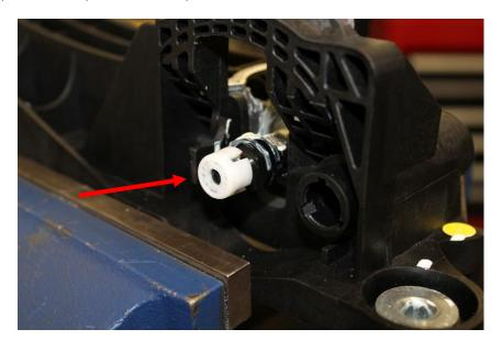
20. Replace the spring removed in step 14 one prong at a time. Put the bottom prong in the top groove of the shifter peg. Then, push the bottom prong down and over the shifter peg and in to the groove.
