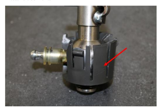
17. Clean the shifter cup of any old grease a debris as well as the shifter socket in the base of the shifter. Apply lithium grease liberally to the ball of your new short shifter, in the end of the ball, in the cup and in the socket of the base.
