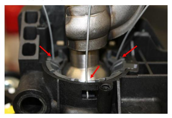
16. Once the tabs are depressed and the wire or paper clips are in place holding the tabs out, pull straight up on the shifter to remove it from the shifter base. Now remove the cup from the bottom of the OEM shifter.
