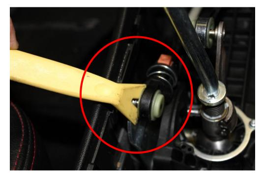
6. Using a window molding removal tool, or a pair of needle nose pliers, or two flat head screw drivers, carefully pop of the shift cable shown below.
