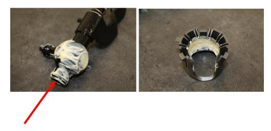
18. Place the cup on the end of your new short shifter. Line up the tabs of the cup with the base and reinsert the shifter in to the base until you hear it snap in.
