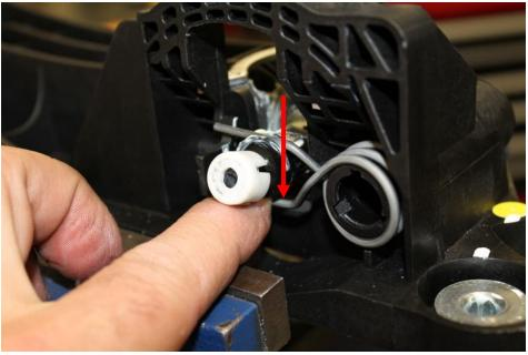
21. Put the cable arm back through the base of the shifter and make sure the points on the arm properly index with the base.
