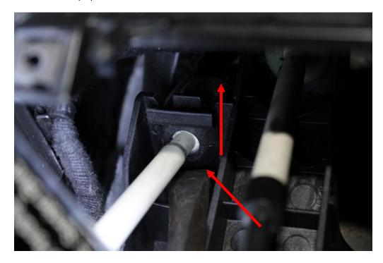
9. Using a 10mm socket remove the 4 bolts that secure the shifter base to the floor of the car. Remove the entire shifter assembly from the car.
