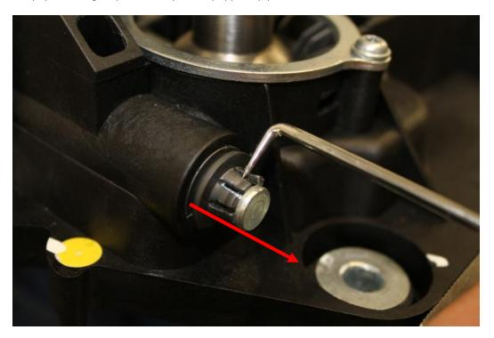
11. Now slide the cable arm out of the base of the shifter.
