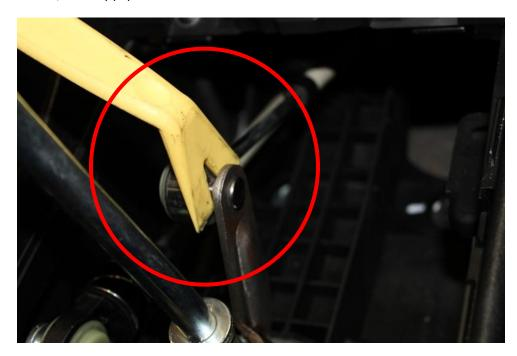
7. Using a large screw driver under the lip of the cable attachment clip, pop the right cable attachment clip up to remove it from the shifter base.
