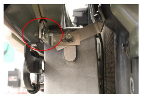
21. Make any necessary adjustments to the intercooler and power steering cooler brackets to ensure there is no contact between the power steering cooler fins and the intercooler.
