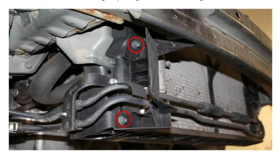
12. Using a 10mm socket, remove the passenger and driver's side power steering cooler mounting brackets.
