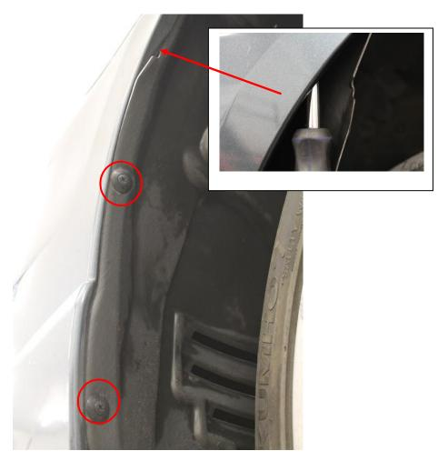
4. Remove two philips head bolts and all push pins securing the top portion of the bumper cover.
