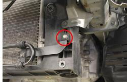
13. Using a 10mm socket, remove the passenger side bracket from the power steering cooler.
