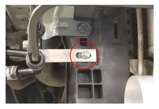
20. Now, attach the driver's side of the power steering cooler to the mounting bracket installed in step 16. Use a bolt removed in step 12, along with 6mm nut and flat washer included with your kit.
