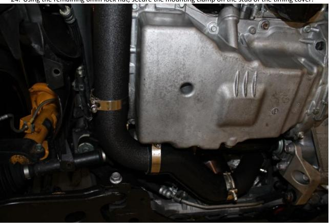
25. Install the hot side core hose using two 2.5" T-bolt clamps. Snug but do not tighten the clamps.
