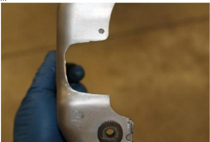
16. The OEM boost controller or any other boost controller can be attached to the upper coolant hard line mounting tab and the vacuum line re-attached to the actuator.
