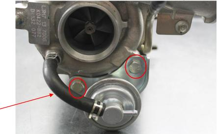
2. Using a pair of needle nose pliers remove the c-clip holding the actuator rod on to the waste gate pivot arm. Do not lose this clip.
