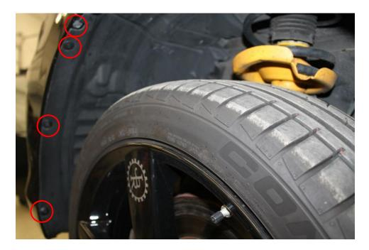
4. Remove two philips head bolts and all push pins securing the top portion of the bumper cover.
