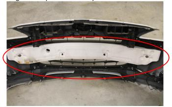
Dry fit the bumper cover and check the two areas circle in **red** below for clearance. If they are close or there is contact with the silicone hoses, the rib of the bracing must be removed. A razor knife or Dremel tool is perfect for this. There may also be some interference with the wiring harness in the areas circled in **green**. Unclip and remove the harness straps if this is an issue.
