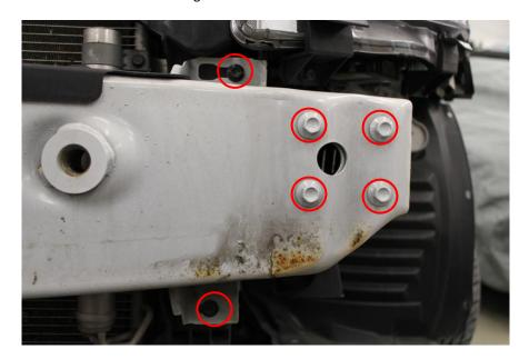
9. Next, install you new JBR Crash Bar and secure it with four of the 14mm bolts removed in step 8 and the four 10mm bolts also removed in step 8. Also use the four spacers and four 17mm bolts included with the kit to secure the crash bar. Tighten the 10mm bolts to 12ft/lbs and the 14m and 17mm to 45ft/lbs.
