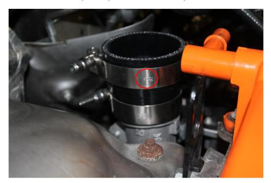
15. Assemble the hot side piping and 90 degree elbow as shown using two 75/67mm T-bolt clamps. Don't worry about getting the clamps too tight at this time. Adjustments will need to be made later.
