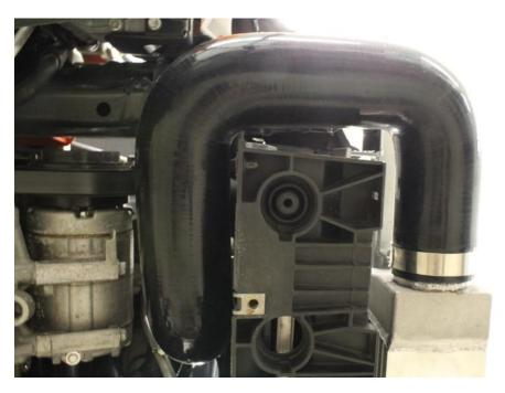
20. Next, put a 75/67mm T-bolt clamp on the intercooler end of the cold side silicone hose and an 81/73mm T-bolt clamp on the throttle body end. Now, feed the cold side silicone hose up from below the car, under the upper radiator hose and on to the throttle body. Tighten the clamp on the throttle body and leave the clamp on the intercooler loose for now.
