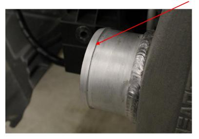
19. Install the U-shaped silicone hose on to the intercooler and on to the polished hot pipe using two 75/67mm T-bolt clamps on each end. Do not tighten them yet.
