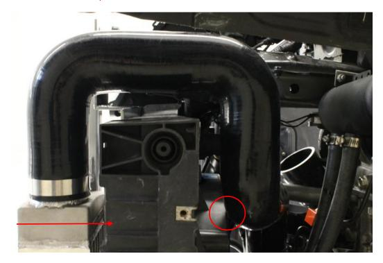
> Bend the ground strap tab down if clearance here is an issue
