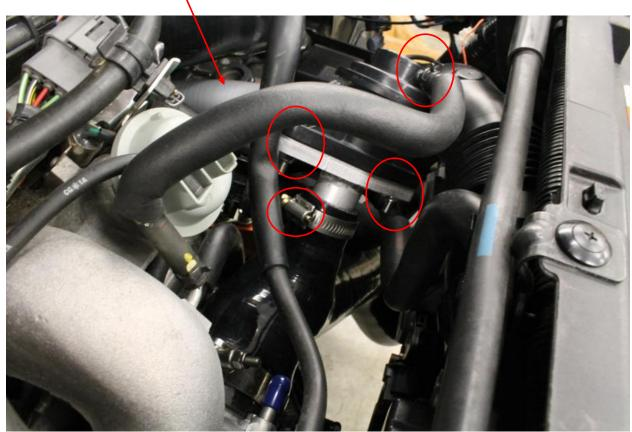
Now let's make some adjustments to ensure there is no rubbing of the silicone hoses. Failure due to rubbing is NOT covered under warranty.
