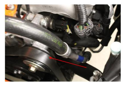
18. Install the hot side piping by dropping the polished pipe down in front of the radiator to the driver's side of the stud that secured the OEM intercooler. Slip the cross over pipe in to the coupler on the turbo. Do not tighten the clamp at the turbo yet. Raise the upper coolant hose running from the coolant reservoir to make room for the 90 degree elbow.
