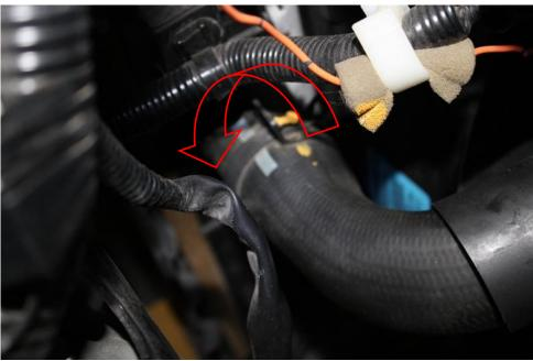
The intercooler core can also be pivoted back a bit if necessary to make sure there is no contact. See the areas circled below for spots to check on the cold side.
