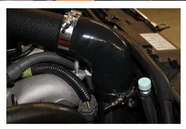
The inlet and outlet of the TR8 Cores we installed had very, very sharp bead rolls machined in to them. These will cut the inner layers of the silicone hoses if this is not addressed. Use a file to soften the inner edge of the bead roll.
