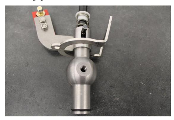
16. Using a crescent wrench tighten the selector arm actuator on to the shifter ball.
