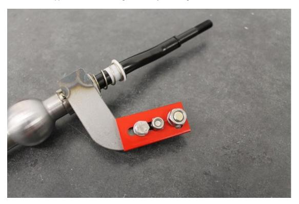
15. Install the gate guide over the base of the shifter as shown.
