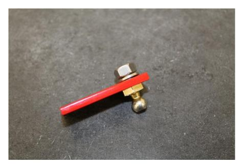
14. Assemble the adjuster plate on to the arm of the shifter using two 6mm bolts and two 6mm nuts oriented opposite of each other. Tighten the adjuster using a 10mm wrench and 10mm socket.
