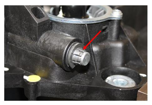
The next two steps are optional but recommended. Performing them will prevent a possible ringing sound from the gate guide while shifting from 1<sup>st</sup> to 2<sup>nd</sup> gear. It will prevent any possible lifting of the gate guide when disengaging from reverse. It also makes the assembly much more solid.
