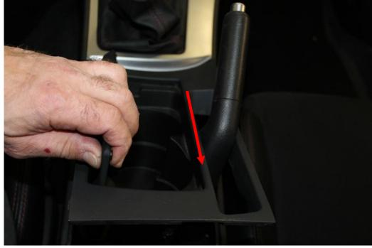
3. Remove the shift boot surround by lifting from the rear, lifting it up and over the shifter then, lay it off to the passenger side of the console.
