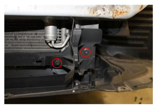
7. Remove the OEM Ambient temperature sensor from the lower portion of the radiator support and relocate it to the hood latch. Re-secure it with a zip tie or electrical tape.
