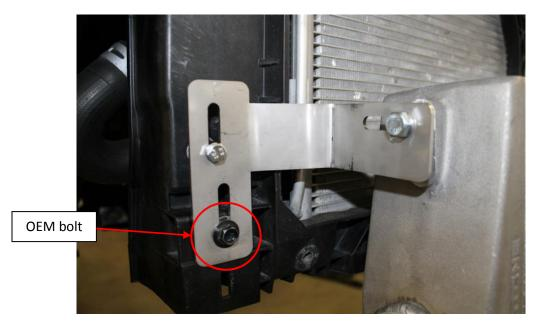
9. Place the nylon spacer behind the bracket Use the 6mm x 1.0 x 35mm bolt, lock washer and flat washer.
