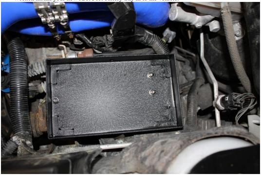
8. Place the included J-hooks through the holes in each side of the battery tray as shown and install your 51R battery.
