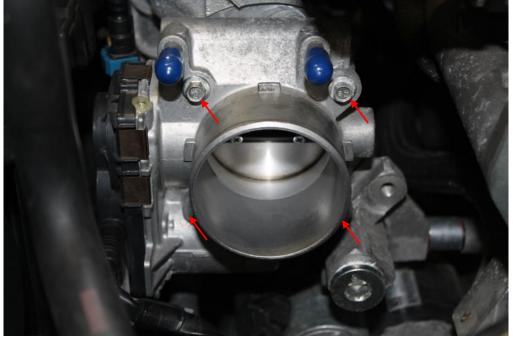
3. Put some Teflon tape or thread sealant on to all the plugs you plan to install in to your spacer and tighten with a 3/16" allen wrench or allen socket.
