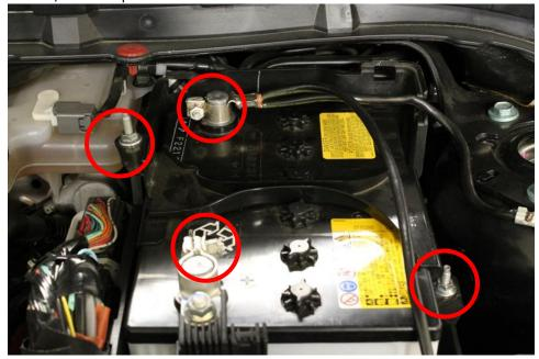
4. Using a pair of needle nose pliers remove the fasteners securing the wiring harness to the front cover of the battery box. There are two on the outside and one inside. Slide the front cover of the battery box up and remove from the vehicle. Remove the battery.
