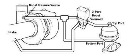
**Important to note!!** You MUST properly tune for the installation of a 3-port EBCS. Using an off-the-shelf tune will result in overboosting!
