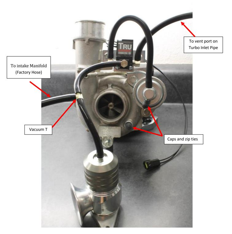
13. Using the included vacuum hose, and vacuum T for 3-Port mode, external waste gate.
