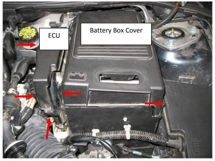
3. Using a 10mm socket, remove the battery hold down bracket, the negative battery terminal connection, then the positive connection.
