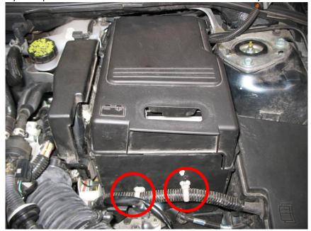
5. Remove the three 10mm bolts in the bottom of the battery box.
