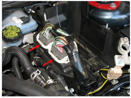
7. Remove the electrical connection to the OEM EBCS and the two vacuum connections. Using a 10mm socket remove the nut securing the OEM EBCS and remove it from the car.
