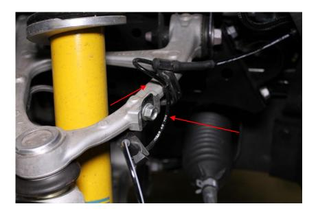
2. Using a 17mm wrench, remove the two bolts securing the upper control arm.
