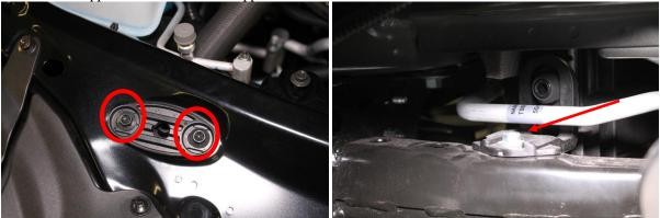
19. Remove the bolt securing the A/C line to the fan shroud with a 10mm socket and detach the wiring harness from the shroud.
