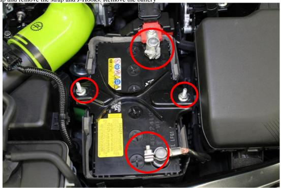
9. Using a 12mm socket, remove the 3 bolts securing the battery tray.
