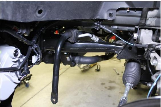
28. Slide the bar towards the driver's side; lift the passenger side arm over the sub-frame.
