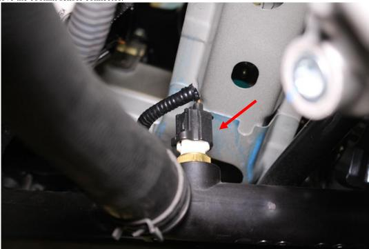
7. Unclip the coolant sensor wire from the sensor housing with a pair of needle nose pliers.
