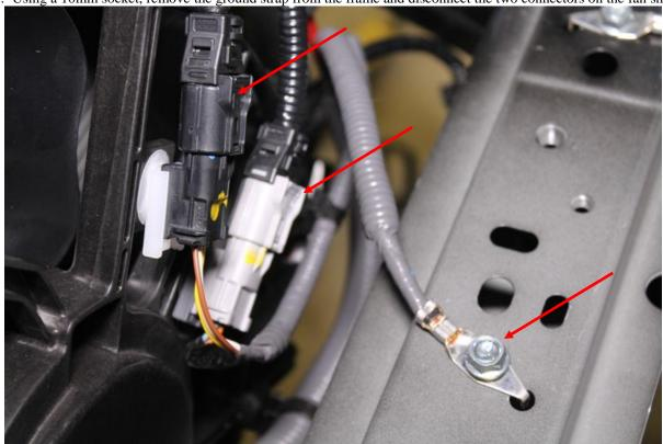
21. Disconnect the wire from the A/C pressure sensor and the other at the shroud.
