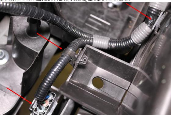
17. Unclip and remove the wiring harness from beneath the core support.
