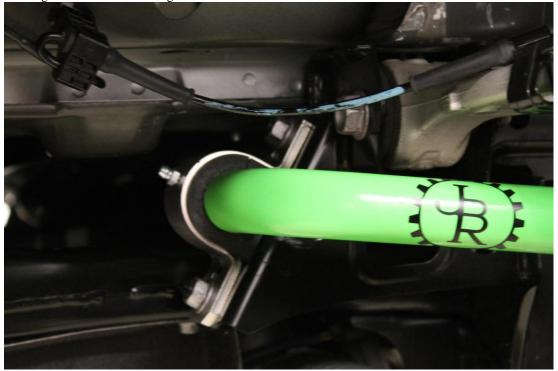
Use only synthetic grease when greasing the bushings. Grease should be applied at each oil change.
