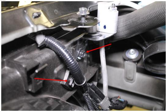
20. Using a 10mm socket, remove the ground strap from the frame and disconnect the two connectors on the fan shroud.
