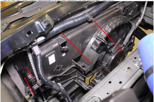
25. Remove the fan shroud by separating it from the radiator on the passenger side, tilting it down and removing it from the bottom of the vehicle. The next series of pictures illustrate the removal. This takes a bit of patience. Be careful not to damage the fins of the radiator.
