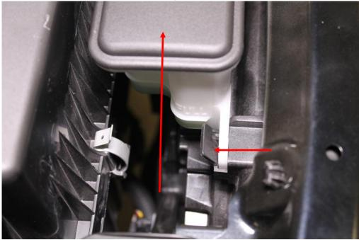
15. Using a 12mm socket remove the air box support bracket.
