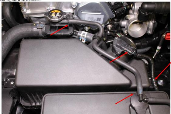
13. Tug up on the entire air box assembly and remove from the vehicle.
