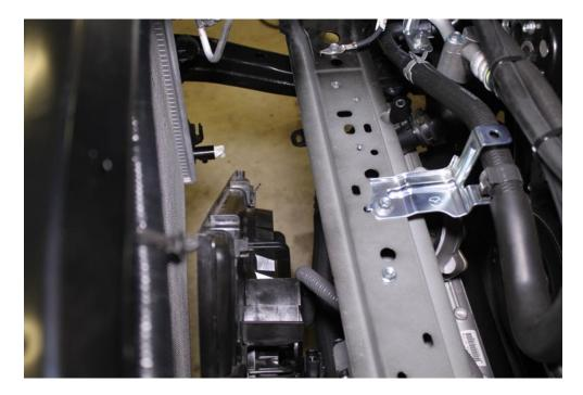
26. Using a 14mm sock and 14mm wrench, remove the 2 nuts from both brackets securing the sway bar to the sub-frame. Remove the brackets.
