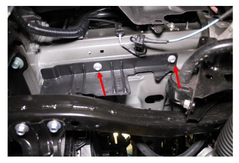
Using a 14mm wrench, remove the nuts securing the endlinks to the sway bar.
