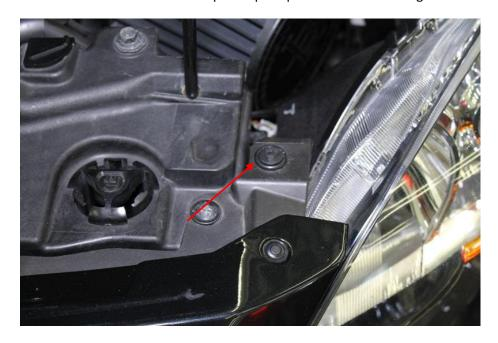
4. Lay your new JBR Radiator Cover in place and secure with the push pins removed in the previous step.
