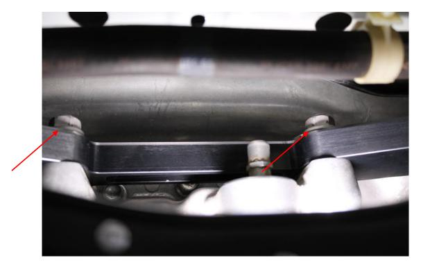
10. Install the two bolts removed in step 7 and tighten to 45 ft/lbs. and reconnect the bracket.
