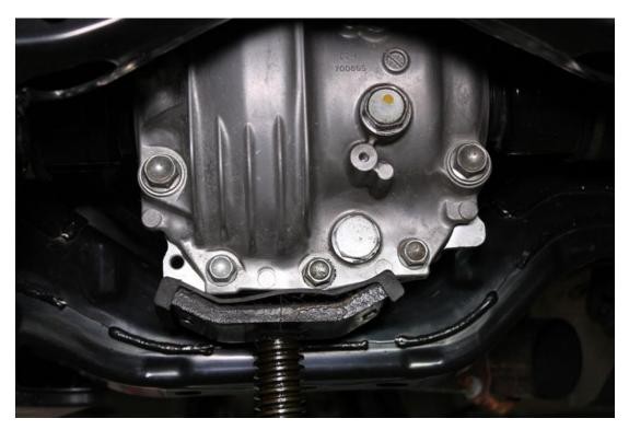
6. Using a 17mm socket and 6" extension, remove the two bolts securing both sides of the OEM differential mount to the sub-frame.
