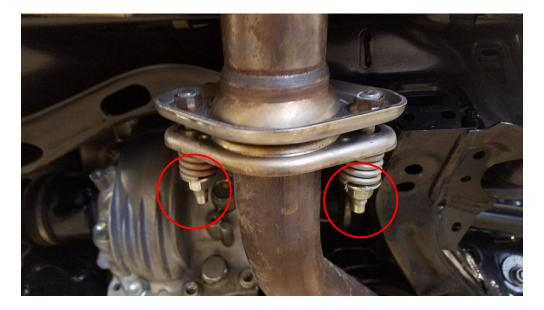
2. Remove the two rubber hangers on either side of the muffler and remove the muffler from the car.
