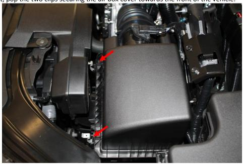
3. Pull the cover slightly towards the front of the vehicle while also raising the cover to expose the OEM paper filter. Reach in and remove the paper filter.
