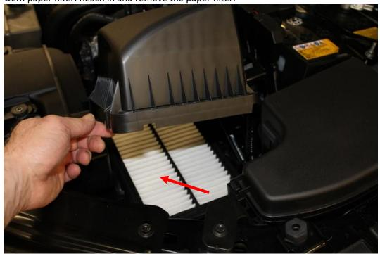
4. After removing the OEM paper filter, install your new JBR Dry FLow Filter in its place. Ensure the rubber seal of the filter is laying properly in the base of the air box.
