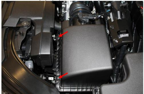
7. Next apply the warning decal to the top of the air box. The top should be clean and dry prior to applying the decal. Using some alcohol will do the trick. Peel the backer of the decal and apply the decal to the top of the air box. Rub it several times to get the decal to adhere and carefully remove the transfer tape.
