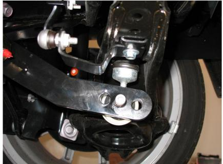
7. Install each of the 4-14mm bolts through the new bushing brackets securing the sway bar to the vehicles sub-frame leaving them loose at this time.
