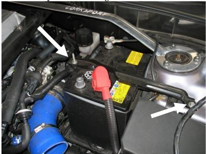
Remove the battery, then remove the battery tray using a 10mm socket and socket wrench
