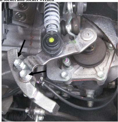
Using needle nose pliers slipped under the shifter cable, pry up to pop the
