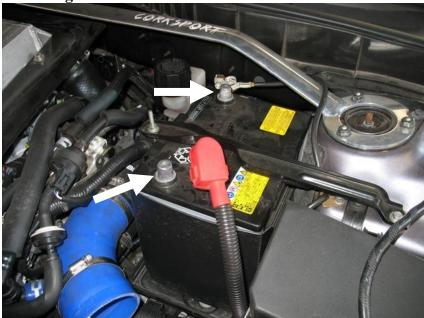
• Remove the battery hold down using a 10mm socket and socket wrench
