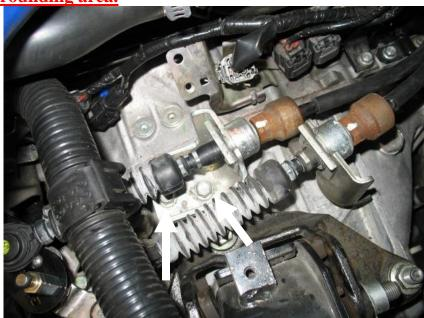
• Insert the 2 provide spacers under the cable mounting bracket as shown below.
