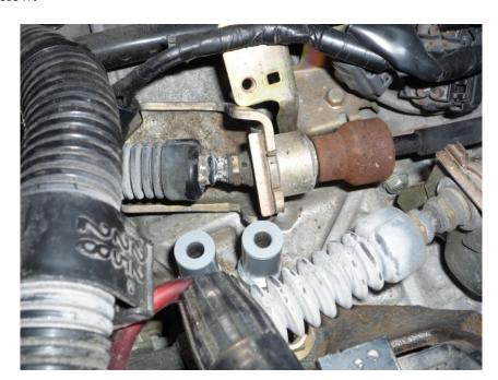
• Apply 1 lock washer 55mm long bolts and re-attach the cable mounting bracket to the transmission and tighten using a 13mm socket and socket wrench (6 point socket is recommended)
