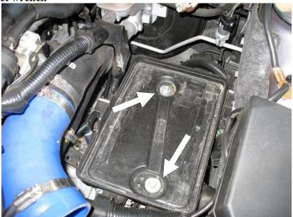
Remove the 2 bolts holding the cable mounting bracket to the transmission with a 12mm socket and socket wrench (6 point socket is recommended)
