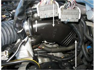
4. Remove 2x 8mm EGR flange bolts and gasket
