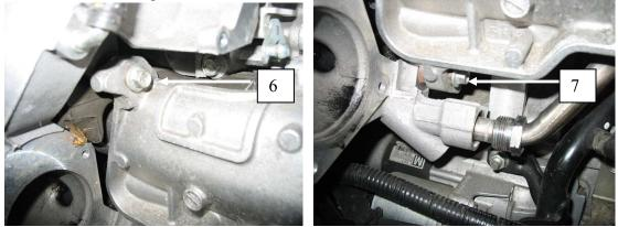
It is highly recommend you re-check and re-torque the intake manifold after a few hundred miles or several heat cycles whichever comes first.
