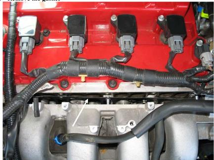
19. Install your new JBR Thermal Intake Gasket the same way the factory gasket was installed
