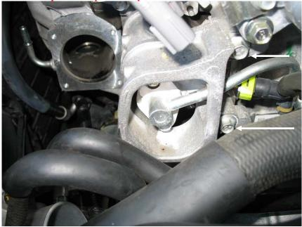
25. Install and torque bolts 6 & 7 to 16FT-lbs
