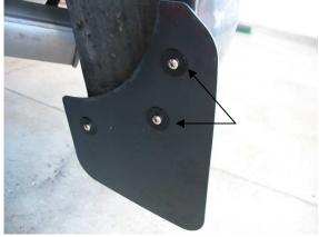
7. Install the 3<sup>rd</sup> long stainless bolt and washer through the mud flap. Place 1 black nylon spacer between the mud flap and the angle bracket. Thread the bolt in to the edge clip that's mounted on the angle bracket and secure loosely. Then tighten all bolts securing the mud flap to the fender using a philips head screw driver ensuring the mud flap is plum and level to the side of the vehicle and the ground.
