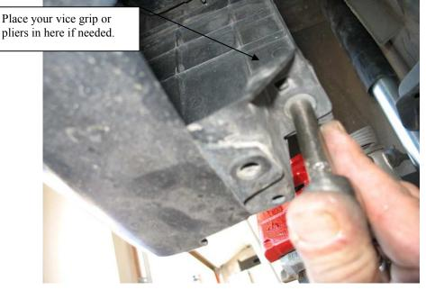
4. Assemble 1 angle bracket with 1 edge clip. Place the edge clip on the slotted side of the angle brake with the angle bracket facing the front of the vehicle and the thread side of the edge clip on the rear side of the angle bracket. Install the angle bracket and edge clip assembly using the bolt removed in the previous step.
