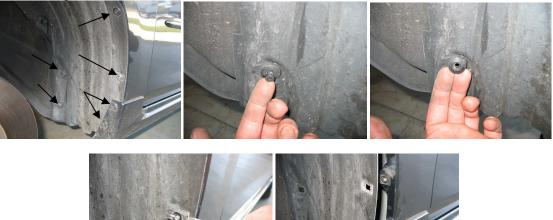
3. Place 2 edge clips over the lowest two holes of the fender liner and one on the tab of the fender.
