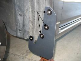
7. Use a scribe or sharp punch to pierce the inner fender liner in the center of the 4<sup>th</sup> mounting hole. Then use the drill & <sup>1</sup>/<sub>4</sub>" drill bit to drill a hole in the inner fender liner.
