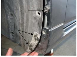
4. Re-install the liner as it was prior to removal. The clips may move during the installation of the liner. To center them us a philips head screw driver or punch.
