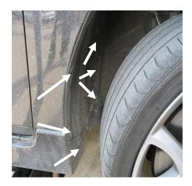
3. Pull the fender liner out from behind and away from the fender.
