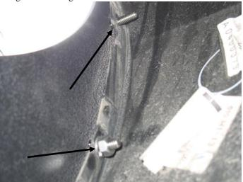
10. Place the 3<sup>rd</sup> bolt and washer through the bottom hole in the mud flap and thread it in to the edge clip on the angle bracket and tighten using a short philips head screw driver.
