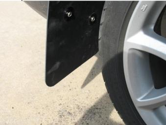
9. From below and behind the bumper place 1 flat washer, 1 lock washer and 1 nut on each of the bolts. Then secure the mud flap to the fender ensuring the mud flap is plum and level to the side of
