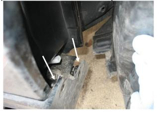
5. Place 1 edge clip over the remaining metal tab in the fender.
