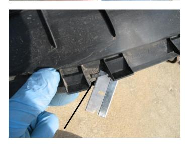
4. Pierce or drill a tiny hole directly in the center of where each of the notches were and then increase the size of the hole using consecutively larger bits until a 1/4" hole is achieved.
