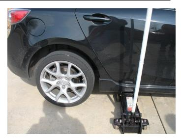
2. Remove all the fasteners securing the inner fender liner from inside the wheel well area and 1 located at the bottom of the bumper and remove the liner from the car.
