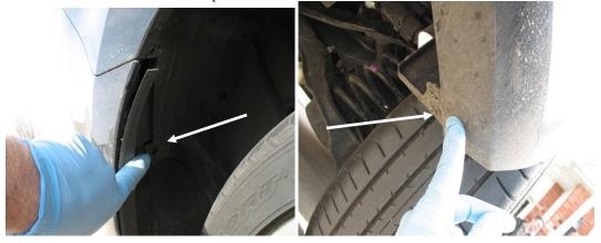
3. Carefully trim off the notches in the fender liner using a sharp razor knife or razor blade.
