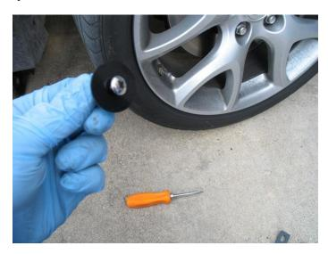
8. Install the front right mud flap with the textured side facing the rear of the vehicle using the 3 bolts and washers. Then secure the mud flap to the fender. Re-install the 3 inner most fasteners for the fender liner.
